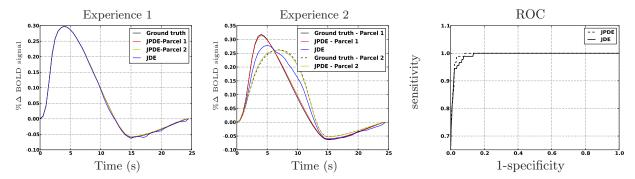
Figure 1: (a): Ground truth and estimated HRFs using JDE and JPDE; (b) ROC curves for activation classification using JDE and JPDE.
