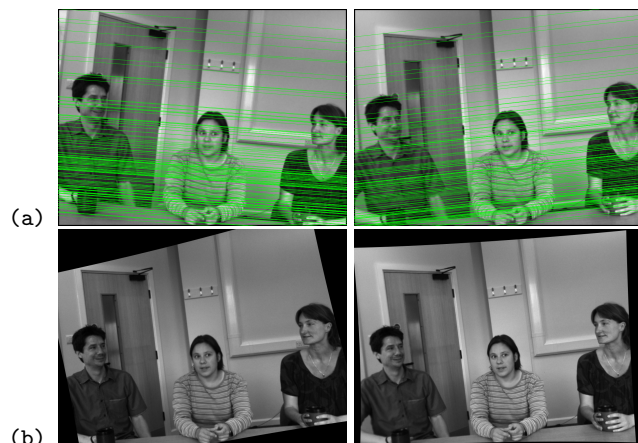
Figure 6: Visual cues: (a) original image pair with superimposed epipolar lines and (b) rectified stereo pair
