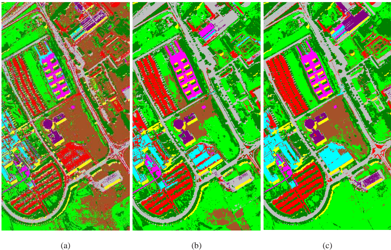
Fig. 7. Thematic map obtained with the University Area: (a) Raw data, (b) EMP_{PCA} , (c) EMP_{KPCA} . The classification was done by SVM with a Gaussian kernel. The color-map is as follows asphalt, meadow, gravel, tree, metal sheet, bare soil, bitumen, brick and shadow.
