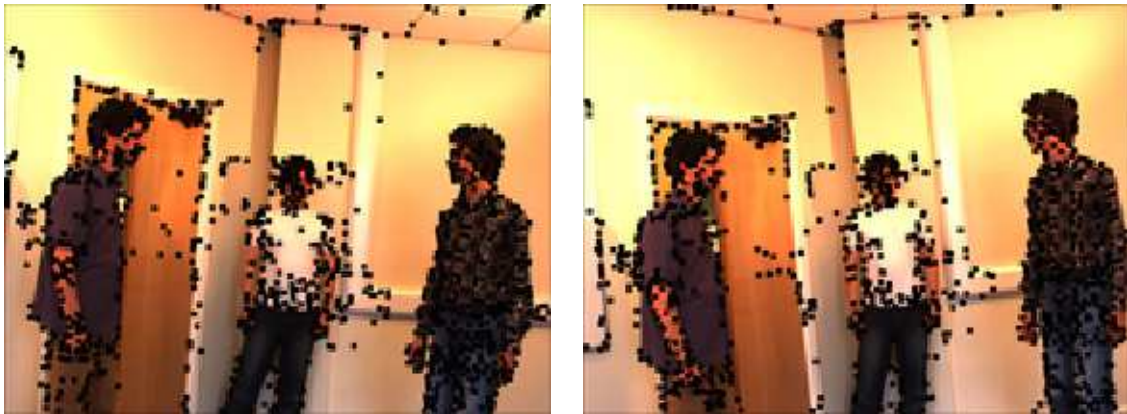
Figure 9: Left and right images corresponding to a frame in a stereo recording with two cameras with the detected interest points in each image. These interest points are then to be matched to produce the 3D data set under consideration.
