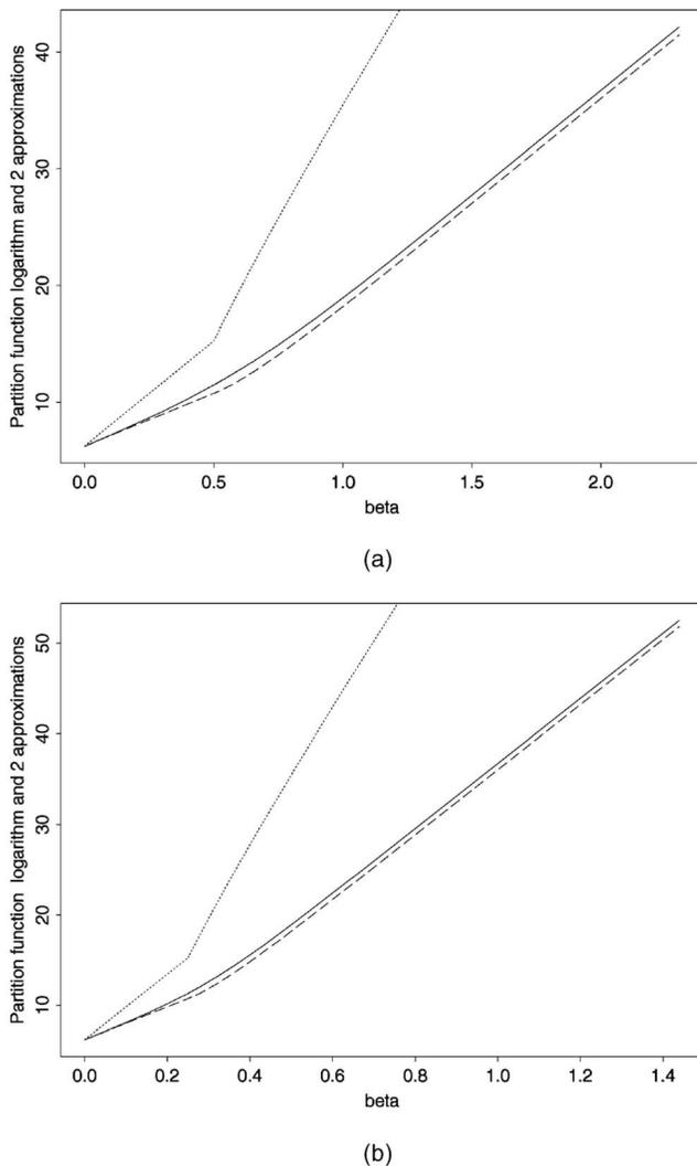
Fig. 5. Two-color Potts model on a  $3 \times 3$  grid with (a)  $N = 4$  neighbors, (b)  $N = 8$  neighbors: exact partition function logarithm and two approximations for  $\beta > 0$ . Solid line shows the exact  $\log W$ , wider dashed line shows  $\log W^{GBF}$ , and smaller dashed line shows  $\log W^{mf}$ .
