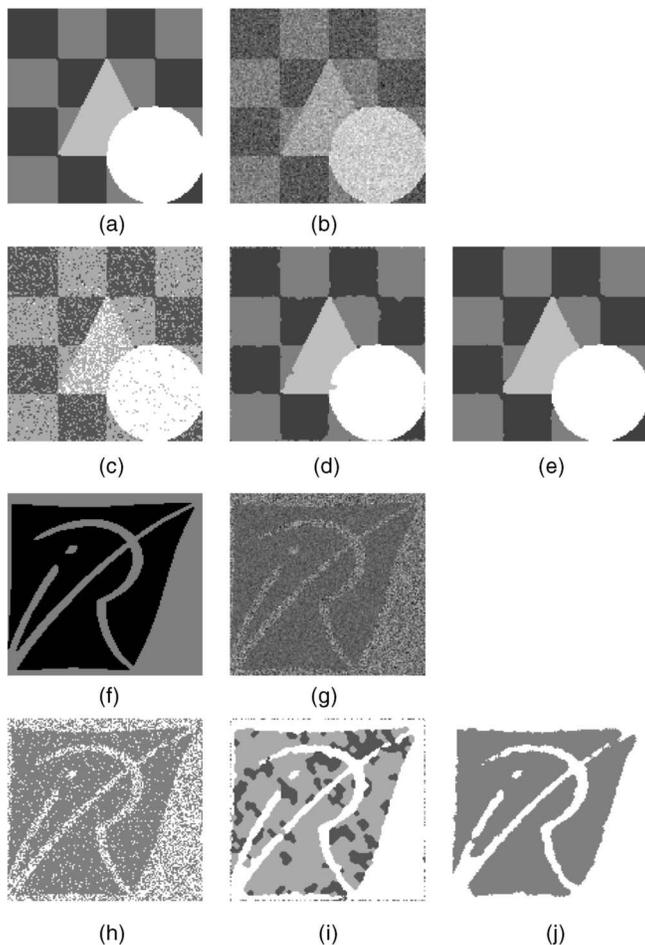
Fig. 2. Noise-corrupted synthetic images. Checkerboard image: (a) original image, (b) noise-corrupted image, (c) 3-color segmentation using EM for independent mixtures, (d) 4-color segmentation using ICM, and (e) 4-color segmentation using the simulated field algorithm. Logo image: (f) original image, (g) noise-corrupted image, (h) 2-color segmentation using EM for independent mixtures, (i) 3-color segmentation using ICM, and (j) 2-color segmentation using the simulated field algorithm.
