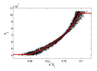
Functional relationship between reduced spectra  $\hat{b}^t X$  on the first GRSIR (PCA+ridge prior) direction and Y, the grain size of CO<sub>2</sub>.
